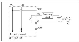
Figure 2. Connecting a Load
